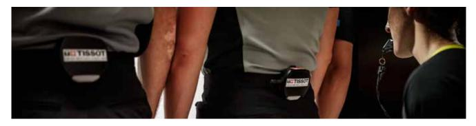
The whistle-controlled time system works via a radio transmitter in the belt pack worn by the officials. Attached to the belt pack is an omnidirectional microphone, which docks in the microphone adapter on the lanyard just below the whistle.
